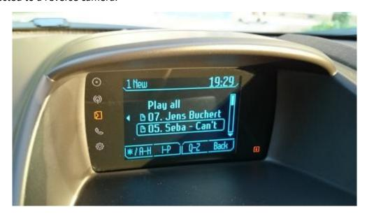
Some later versions of SYNC 1 have a colour screen and can show optical parking sensor information or a reverse camera feed. There are two versions with a colour screen, which effects which parts you need to fit a reverse camera. Either will need coding to recognise a connected reverse camera.
