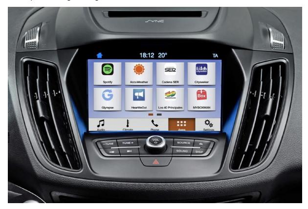
SYNC 3 is now found on a range of vehicles, some have it all built into the screen, while others have a separate module behind the glove box and the screen on the dashboard is only a peripheral input device.
